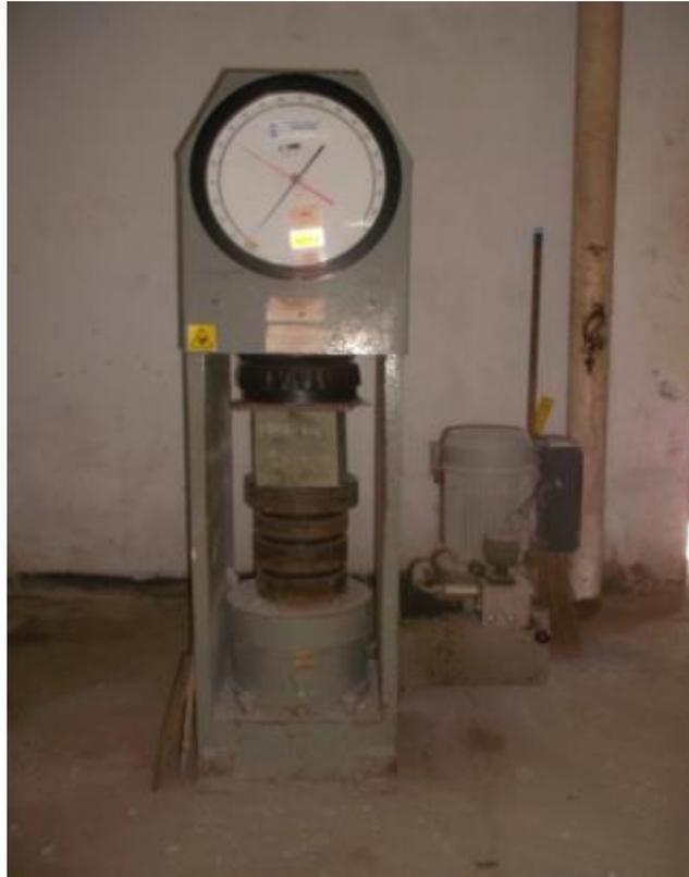
Gambar 2. Alat *Compression Testing Machine* (CTM)
